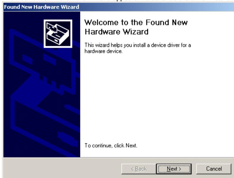
**Note:** On Windows XP systems, the Microsoft Windows CCID Class driver may be activated without showing the **Found New Hardware Wizard**. If this is the case, replace the Microsoft PC/SC driver manually with the OMNIKEY proprietary PC/SC driver using the Device Manager. See Section 9 Appendix C - Manual Driver , page 24.
